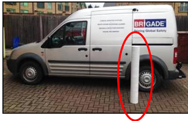
1m long pole below a camera mounted at 1.8m
